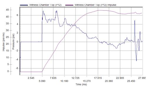
Peak Pressure: 7.15 psi at 8.42 ms Duration: 9.73 ms Test Date: 12/16/2014 Test Time: 9:02 am
