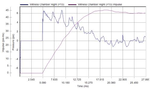
Peak Pressure: 6.74 psi at 9.32 ms Duration: 8.25 ms Test Date: 12/16/2014 Test Time: 1:42 pm
