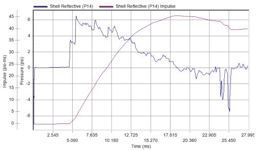
Peak Pressure: 6.53 psi at 5.58 ms Test Date: 12/16/2014 Duration: 13.04 ms Test Time: 4:57 pm
