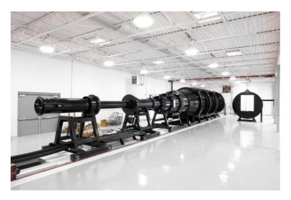
Figure #1 Shock Tube and Test Facility
