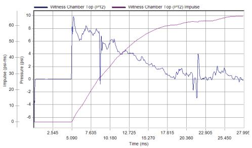
Peak Pressure: 9.94 psi at 5.30 ms Duration: 3.53 ms Test Date: 12/19/2014 Test Time: 10:15 am
