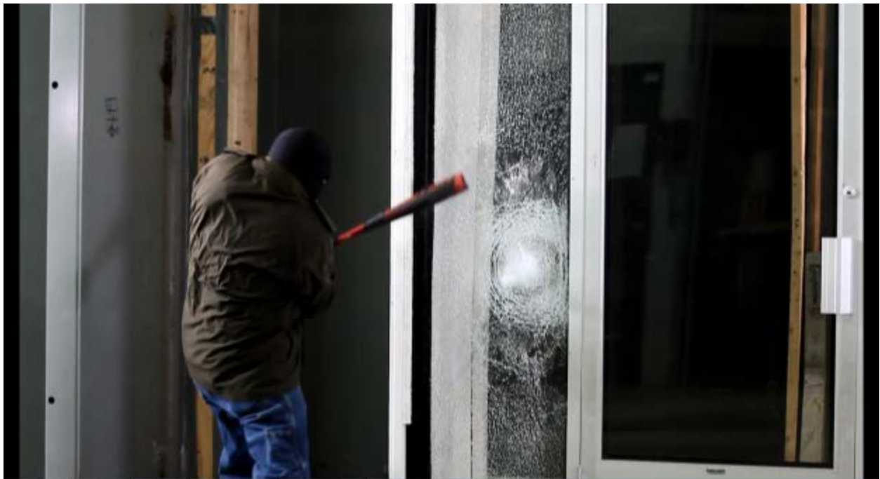
Test #3: Bat attack, 3M Ultra 600.
