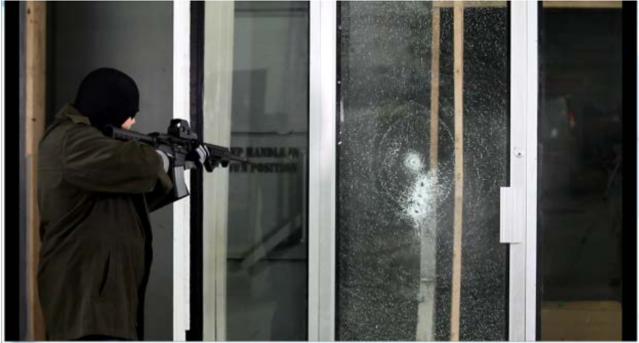
Test #1: Semi-automatic rifle attack, 3M Ultra 600 (interior) with Safety S70 Exterior (exterior).
