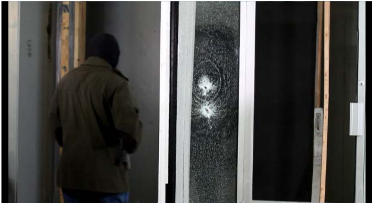
Test #2: Semi-automatic rifle attack, 3M Ultra 600 (interior) with Safety S70 Exterior (exterior).
