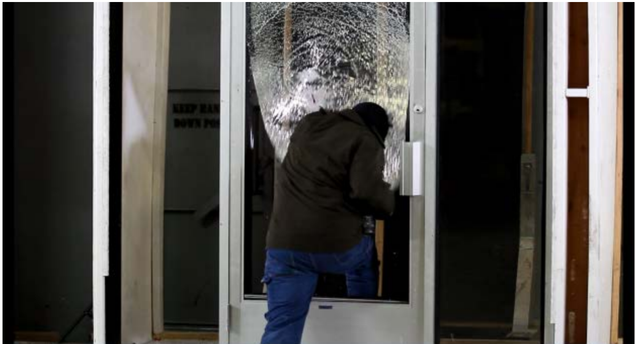
Test #4: Semi-automatic rifle attack, access gained after 19 impacts and 18 seconds (film attachment failed – adhesion to film).
