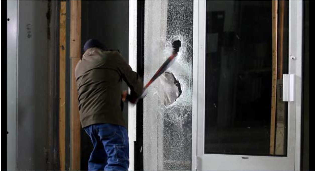
Test #3: Bat attack, 3M Ultra 600, after several impacts,
