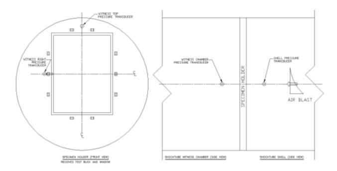
Figure #2 Pressure Sensor Locations
