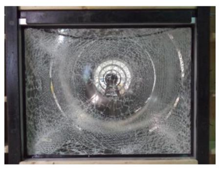
Photo No. 5 Post-test Specimen #2, Interior
