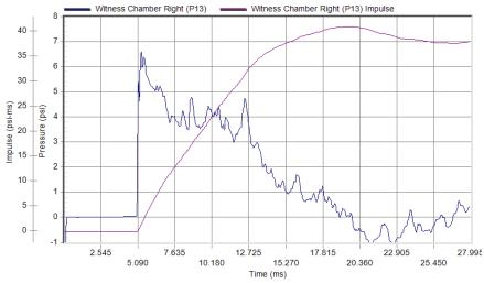
Peak Pressure: 6.58 psi at 5.33 ms Test Date: 10/15/2013 Duration: 13.61 ms Test Time: 11:11 am
