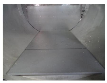
Photo No. 3 Post-test Specimen #1, Witness Chamber
