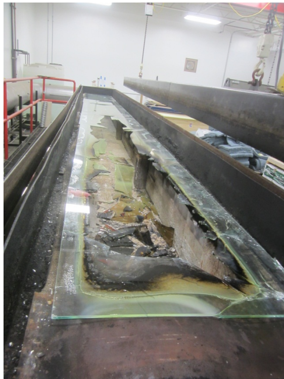
Photo No. 2 Unexposed Surface (Post-test) www.archtest.com
