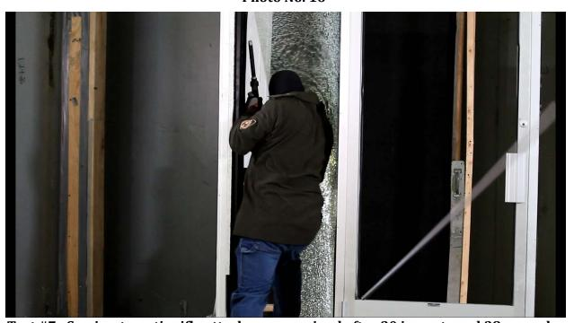
Test #7: Semi-automatic rifle attack, access gained after 30 impacts and 38 seconds.
