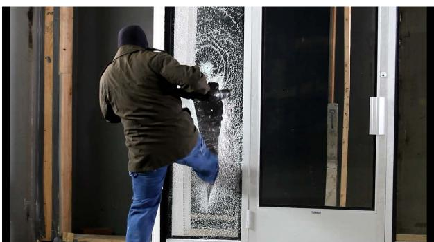
Test #9: Semi-automatic rifle attack, after 38 seconds.
