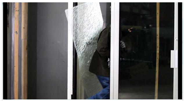
Test #3: Semi-automatic rifle attack, accessed gained after 27 impacts and 27 seconds.
