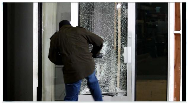
Test #5: Semi-automatic rifle attack, after 45 seconds.
