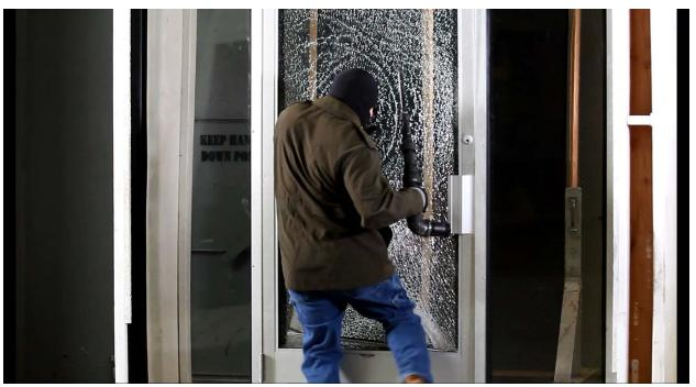
Test #10: Semi-automatic rifle attack, after 70 seconds.
