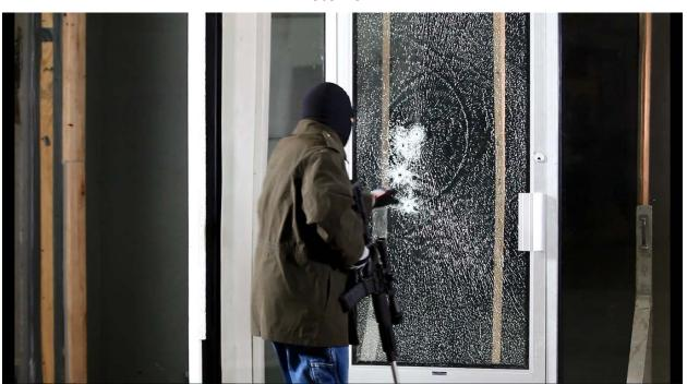
Test #10: Semi-automatic rifle attack, 3M Scotchshield Ultra 800 (interior) with Safety S70 Exterior (exterior).
