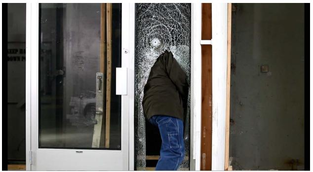
Test #4: Semi-automatic rifle attack, accessed gained after 41 impacts and 43 seconds.
