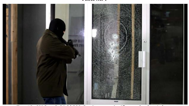
Test #2: 3M Scotchshield 800, Semi-automatic rifle attack, after 4 shots.
