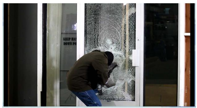
Test #5: Semi-automatic rifle attack, access gained 64 impacts and after 81 seconds.
