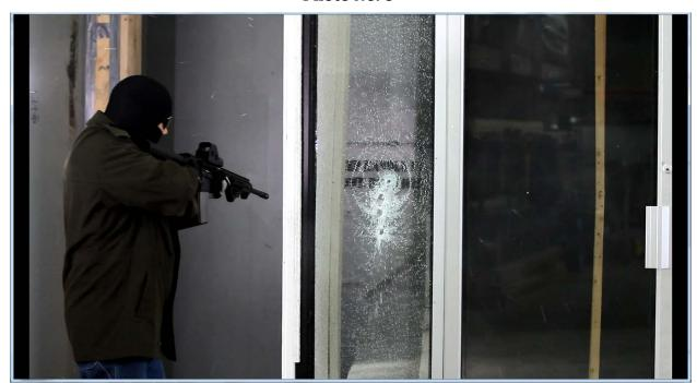
Test #3: 3M Safety S80, Semi-automatic rifle attack, after 4 shots.
