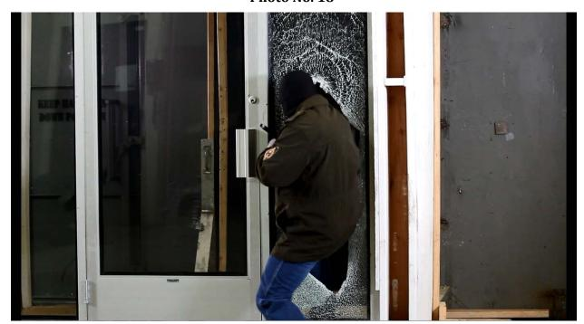
Test #8: Semi-automatic rifle attack, access gained after 45 impacts and 50 seconds.
