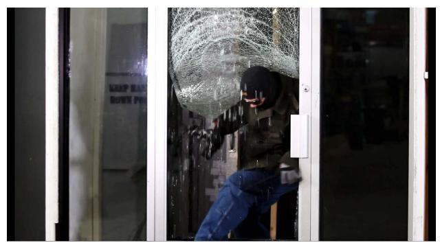
Test #2: Semi-automatic rifle attack, accessed gained after 33 impacts and 35 seconds.
