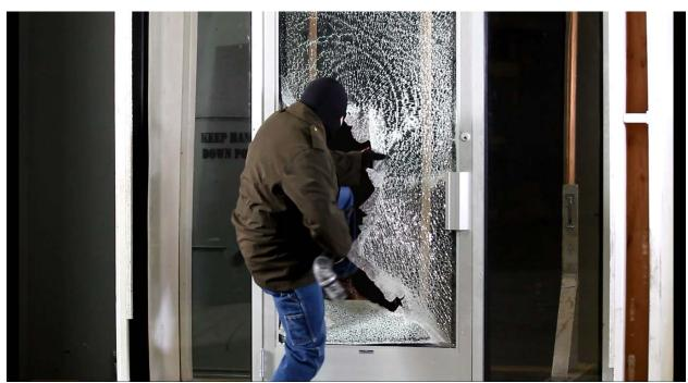
Test #10: Semi-automatic rifle attack, access gained after 70 impacts and 91 seconds.
