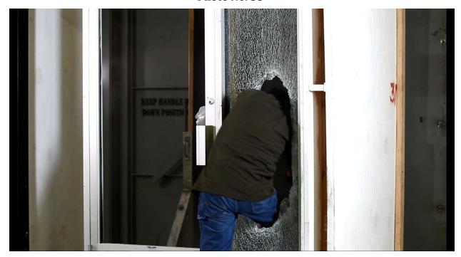
Test #15: Bat attack, 3M Safety S80, access gained after 17 impacts and 16 seconds.
