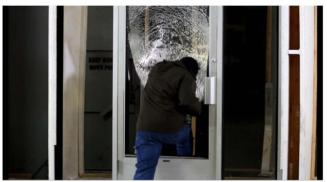
Test #13: Semi-automatic rifle attack, access gained after 19 impacts and 18 seconds (film attachment failed - adhesion to film).
