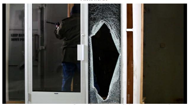
Test #11: Semi-automatic rifle attack, access gained after 25 impacts and 29 seconds.
