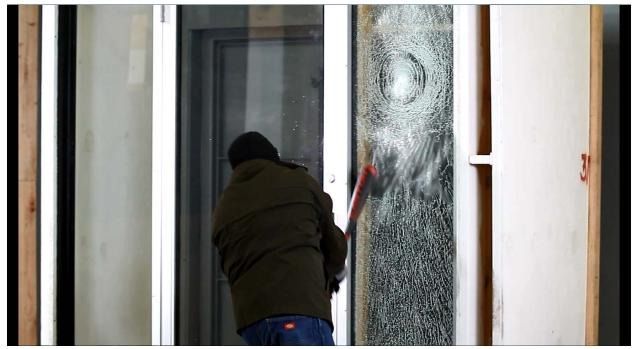
Test #1: Bat attack, 3M Scotchshield Ultra 800 (interior) with Safety S70 Exterior (exterior).
