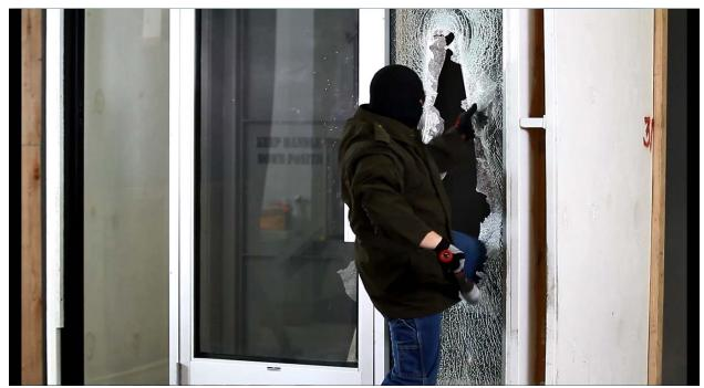
Test #1: Bat attack, accessed gained after 37 impacts and 30 seconds.
