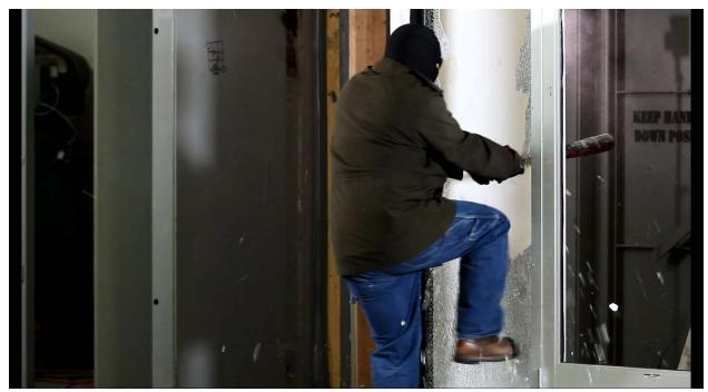
Test #14: Bat attack, NO FILM, access gained in 6 seconds.
