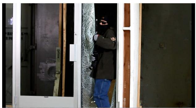
Test #6: Semi-automatic rifle attack, access gained after 38 impacts and 60 seconds.
