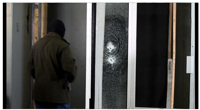
Test #7: Semi-automatic rifle attack, 3M Scotchshield Ultra 600 (interior) with Safety S70 Exterior (exterior).
