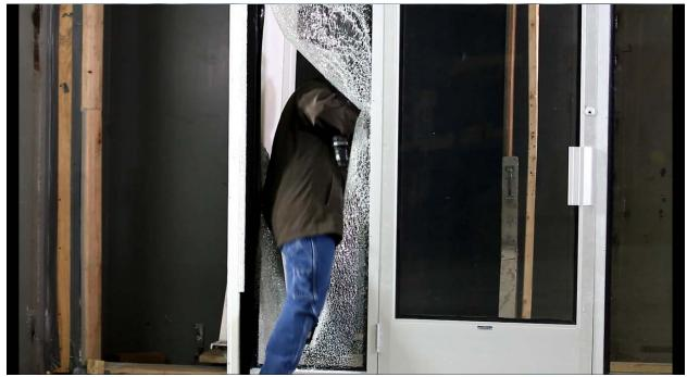
Test #9: Semi-automatic rifle attack, access gained after 43 impact and 48 seconds.
