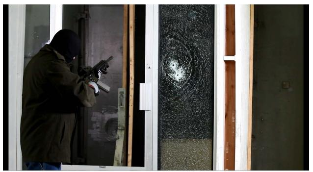
Test #6: 3M Scotchshield Ultra 800, Semi-automatic rifle attack, after 2 shots and jammed gun.
