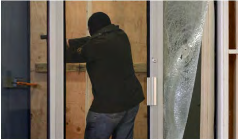
Test #3: Handgun attack, 3M Ultra S600. Access after 30 seconds.
