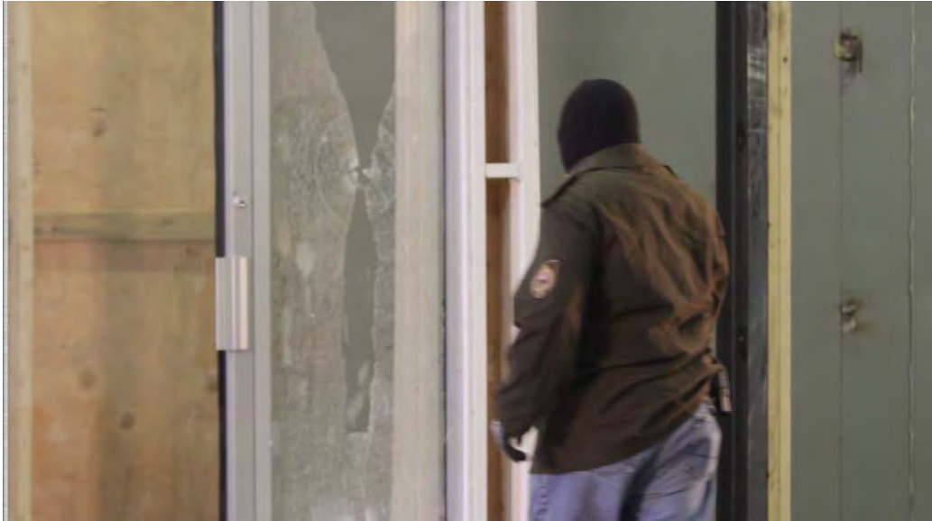
Test #2: Handgun attack, no security film. After 1 gun shot.
