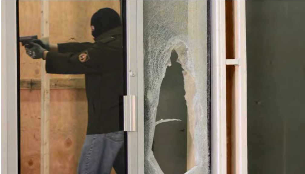
Test #1: Handgun attack, 3M Safety S140 (14-mil Security Film). Access after 4 gun shots, 35 upper body attacks, 39 kicking attempts, 24 impacts with baseball bat. Total time elapsed was 122 seconds.
