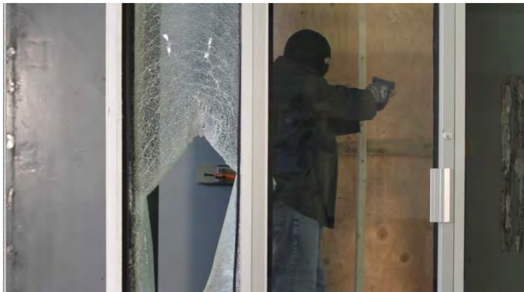
Test #4: Handgun attack, 3M 6-mil microlayered film. Access after 4 gun shots, 11 upper body attacks, 23 kick attempts. Total time elapsed was 58 seconds.
