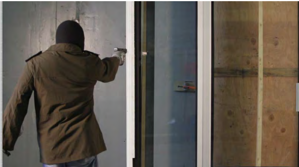
Test #4: Handgun attack, 3M 6-mil microlayered film.
