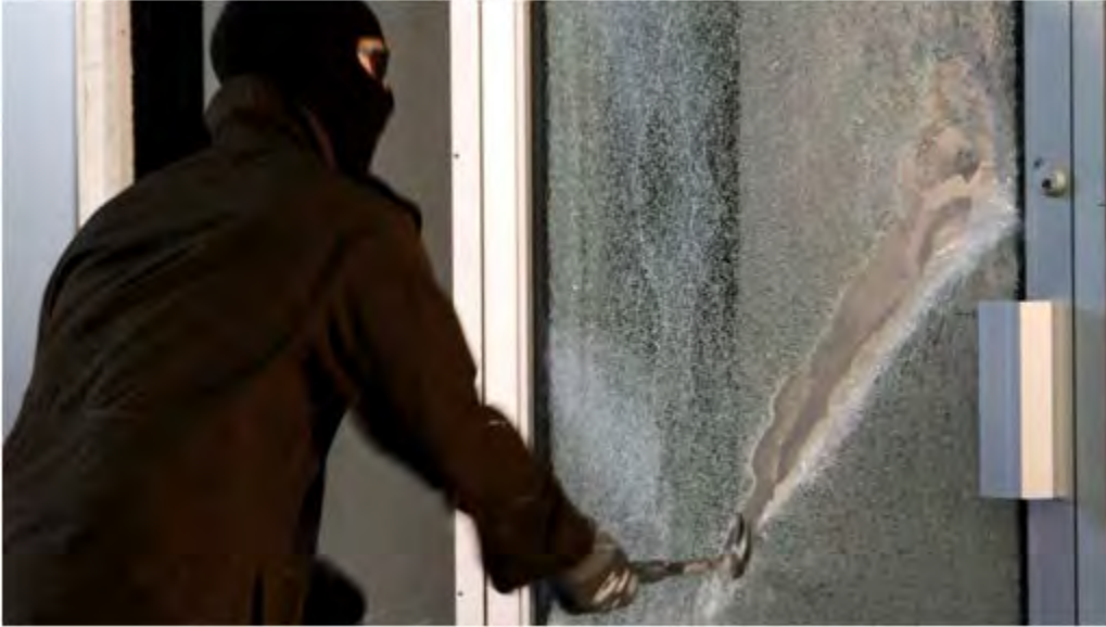
Test #9: Claw hammer attack, 3M 6-mil microlayered film. Continued attack after unsuccessful attempt to unlock door.
