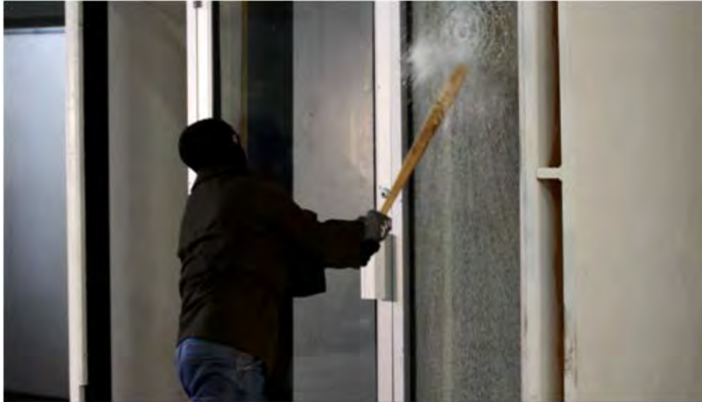
Test #7: Baseball bat attack, 3M 6-mil microlayered film.
