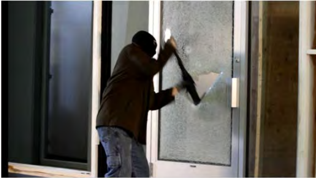
Test #5: Semi-automatic rifle attack, 3M Safety S140 (14-mil Security Film). Simulated rifle attack, using 9-lb steel pipe.
