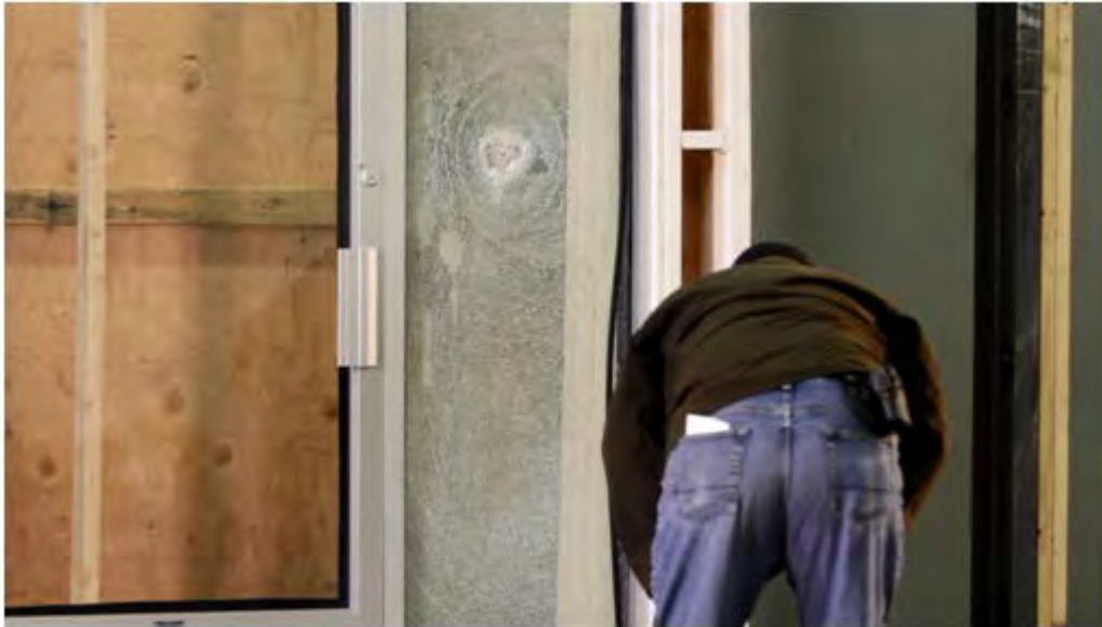
Test #1: Handgun attack, 3M Safety S140 (14-mil Security Film). After 4 gun shots, 35 upper body attacks, 39 kicking attempts. Total time elapsed was 95 seconds.
