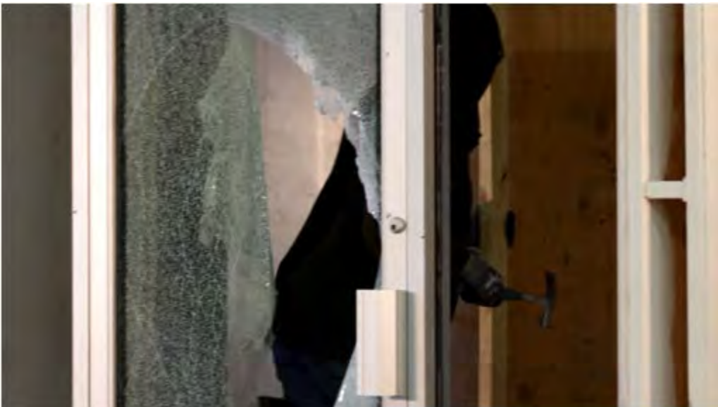
Test #9: Claw hammer attack, 3M 6-mil microlayered film. Continued attack after unsuccessful attempt to unlock door. Access after 33 seconds.
