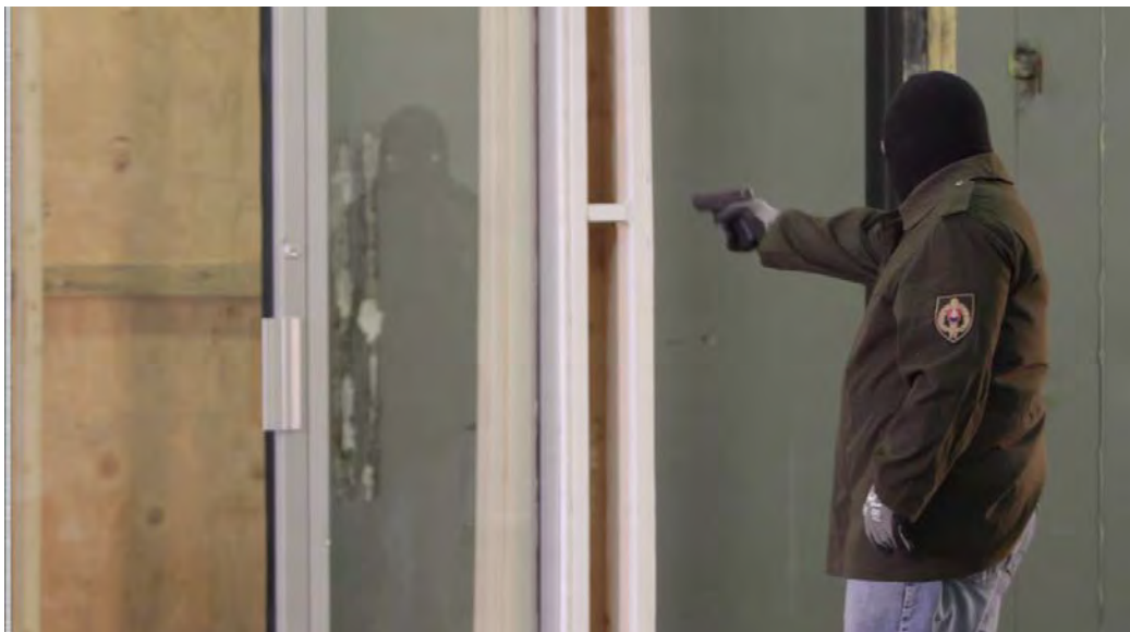
Test #2: Handgun attack, no security film.
