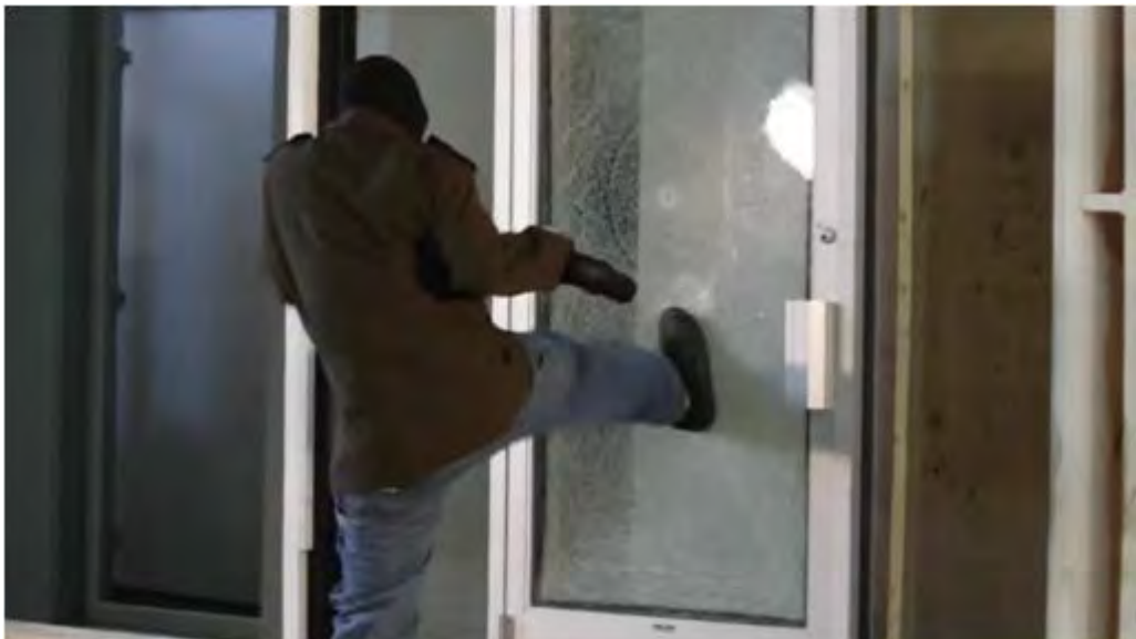
Test #5: Semi-automatic rifle attack, 3M Safety S140 (14-mil Security Film). Kick attempts after 4 gunshots.
