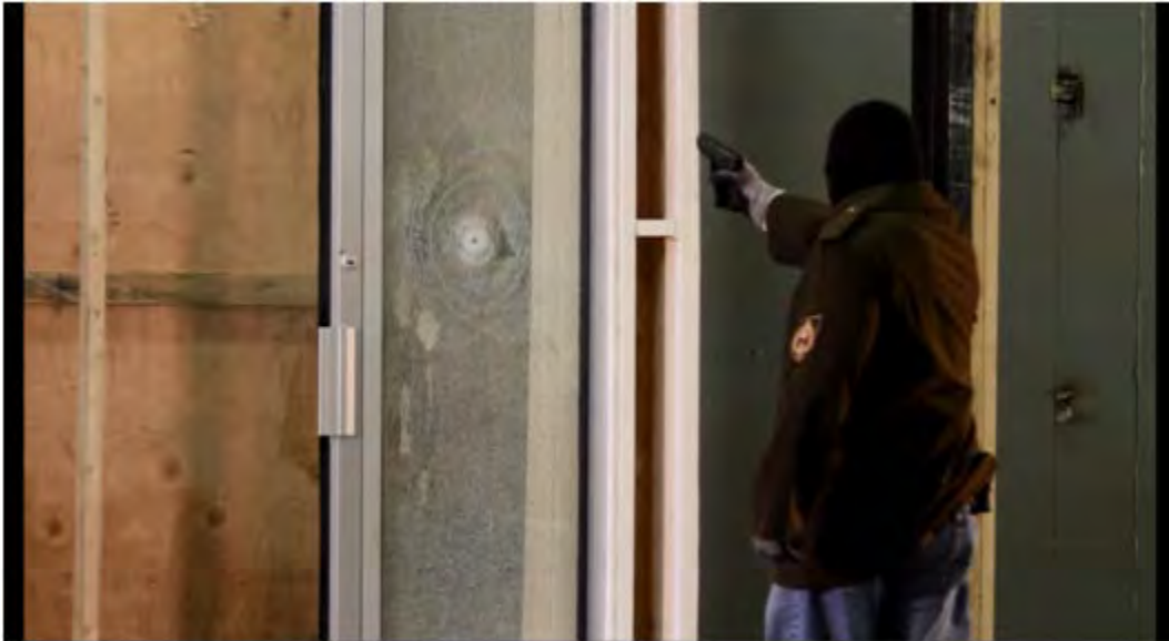
Test #1: Handgun attack, 3M Safety S140 (14-mil Security Film).
