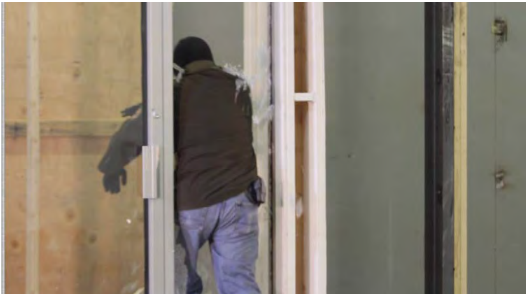
Test #2: Handgun attack, no security film. Access after 3 seconds.
