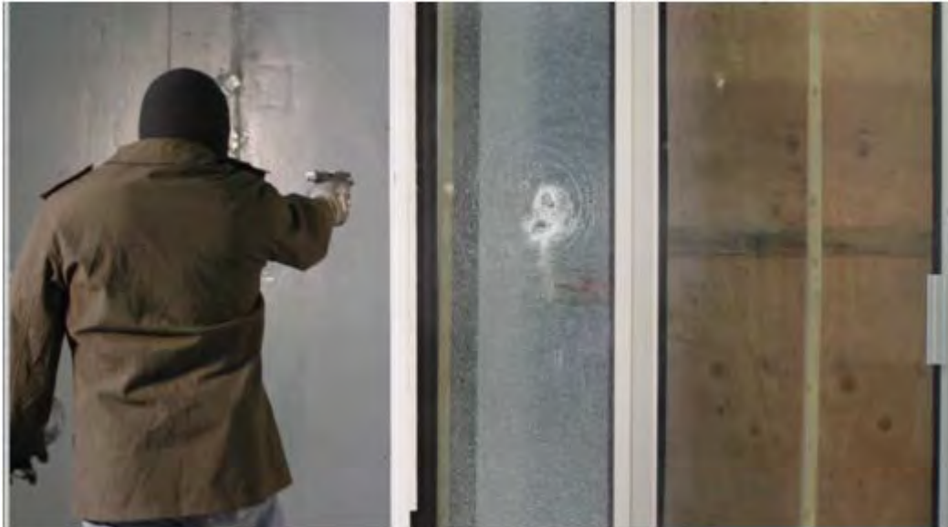
Test #4: Handgun attack, 3M 6-mil microlayered film. After 4 gun shots.
