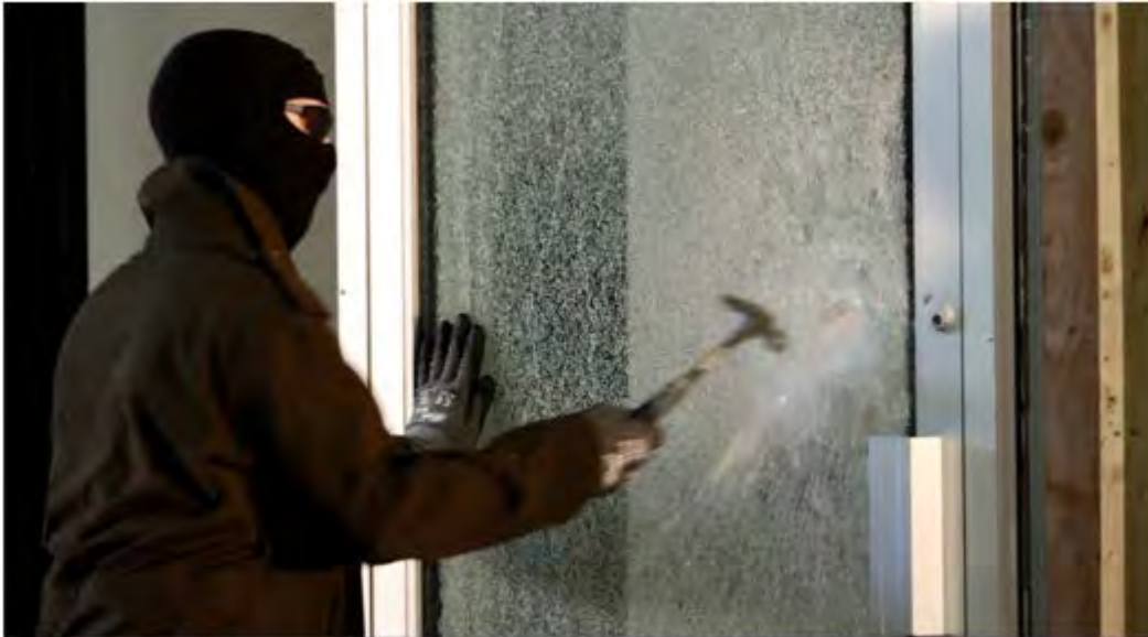
Test #9: Claw hammer attack, 3M 6-mil microlayered film.
