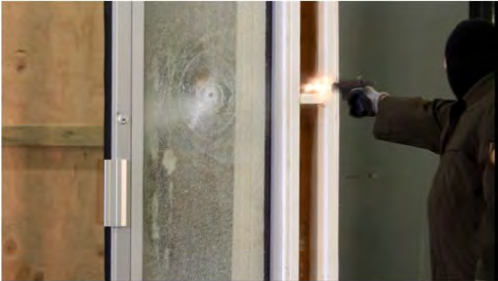
Test #3: Handgun attack, 3M Ultra S600.
