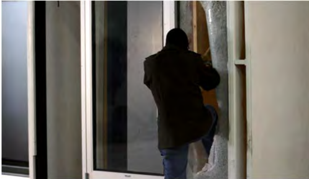
Test #7: Baseball bat attack, 3M 6-mil microlayered film. Access after 28 impacts. Total time elapsed was 28 seconds.
