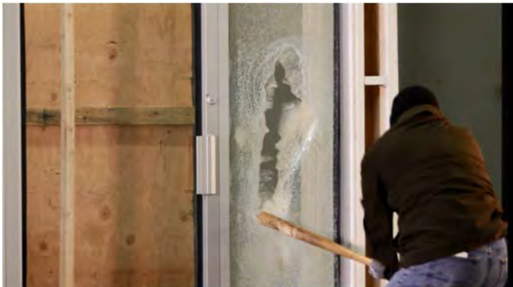
Test #1: Handgun attack, 3M Safety S140 (14-mil Security Film). Attack with baseball bat.
