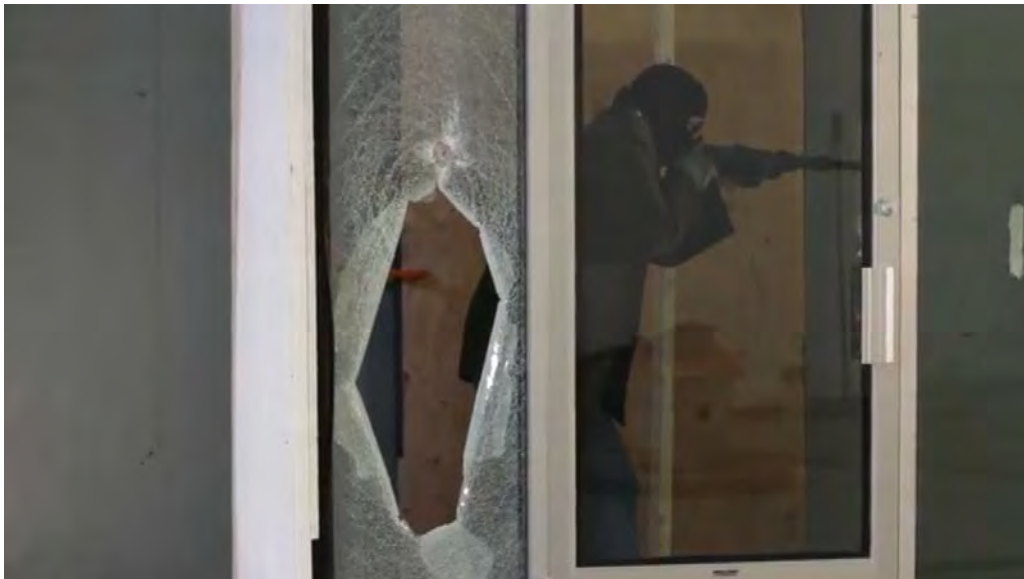
Test #6: Semi-automatic rifle attack, 3M 6-mil microlayered film. Access after 4 gun shots, 12 upper body attacks, 14 kick attempts. Total time elapsed was 44 seconds.
