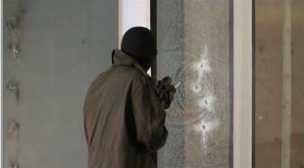
Test #6: Semi-automatic rifle attack, 3M 6-mil microlayered film. After 4 gunshots.
