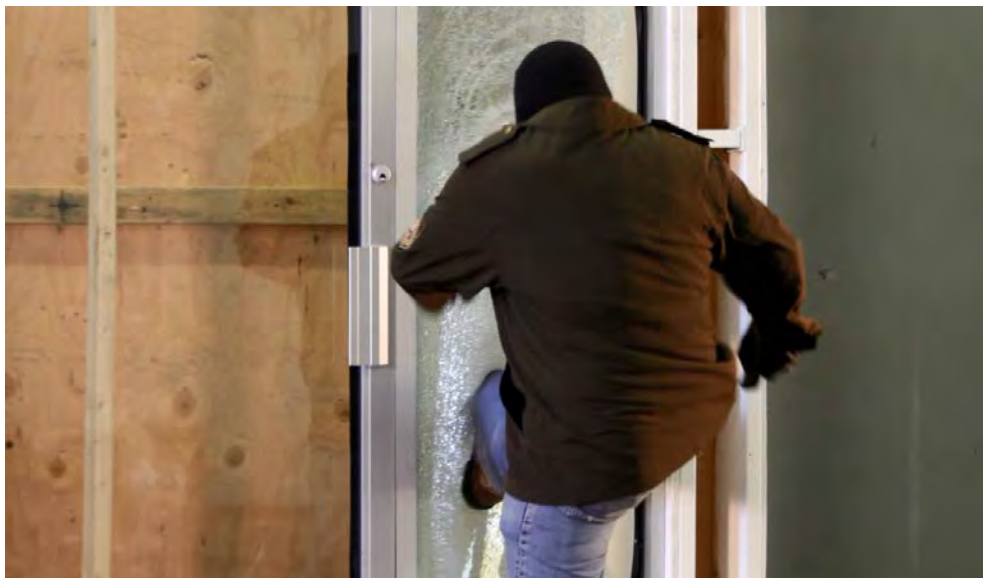
Test #3: Handgun attack, 3M Ultra S600. Attachment System failure in lower right corner at 28 seconds.
