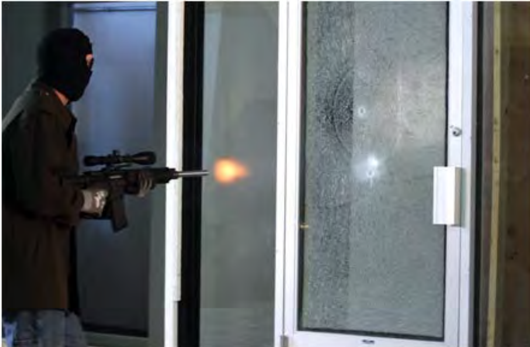
Test #5: Semi-automatic rifle attack, 3M Safety S140 (14-mil Security Film). After 4 gunshots.
