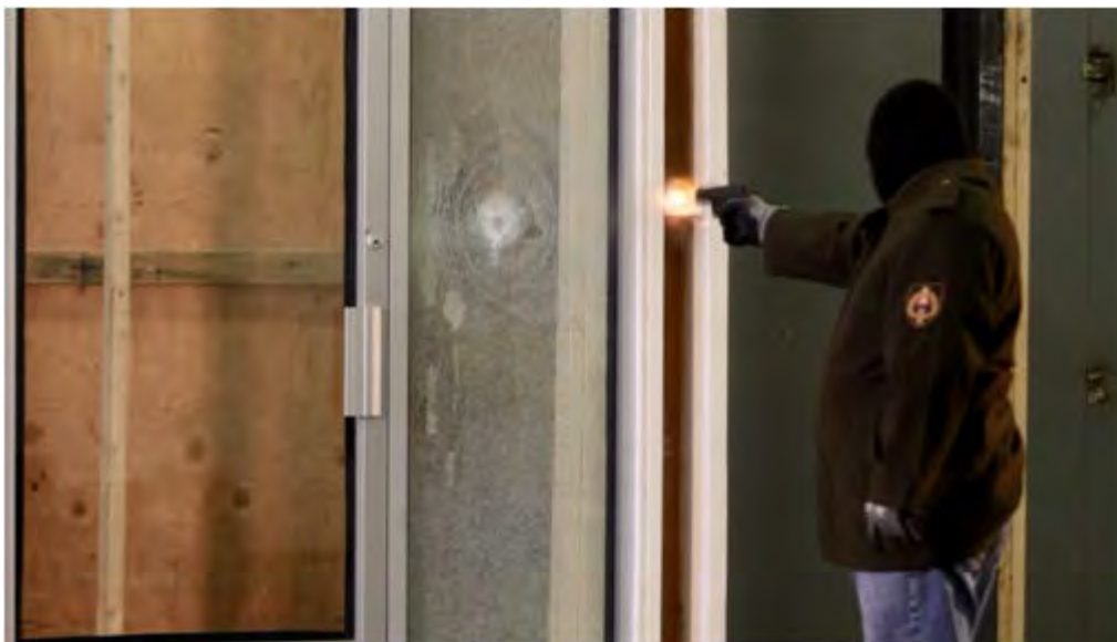
Test #1: Handgun attack, 3M Safety S140 (14-mil Security Film). After 4 gun shots.
