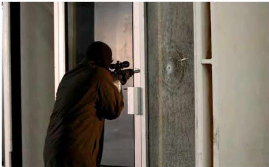
Test #8: Semi-automatic rifle attack, 3M 6-mil microlayered film.
