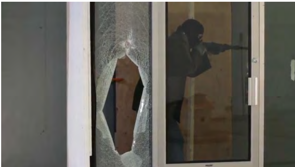
Test #3: Semi-automatic rifle attack, 3M 6-mil microlayered film. Access after 4 gun shots, 12 upper body attacks, 14 kick attempts. Total time elapsed was 44 seconds.
