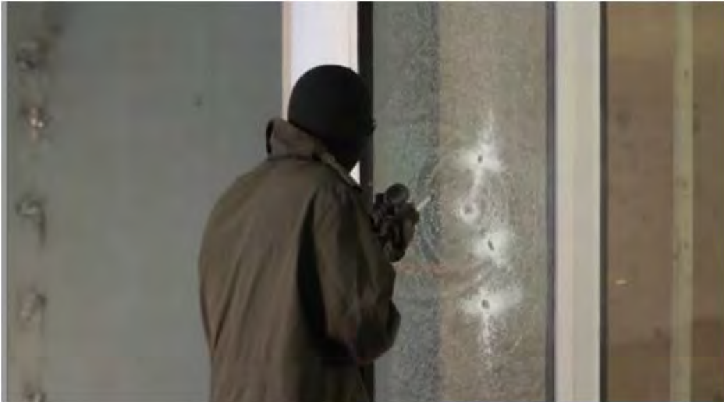
Test #3: Semi-automatic rifle attack, 3M 6-mil microlayered film. After 4 gunshots.
