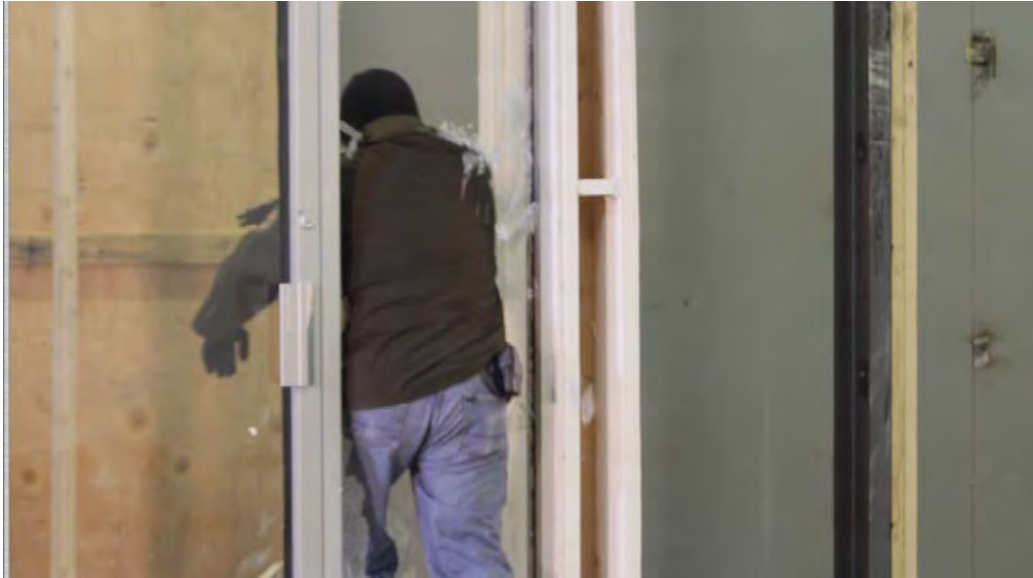
Test #1: Handgun attack, no security film. Access after 3 seconds.
