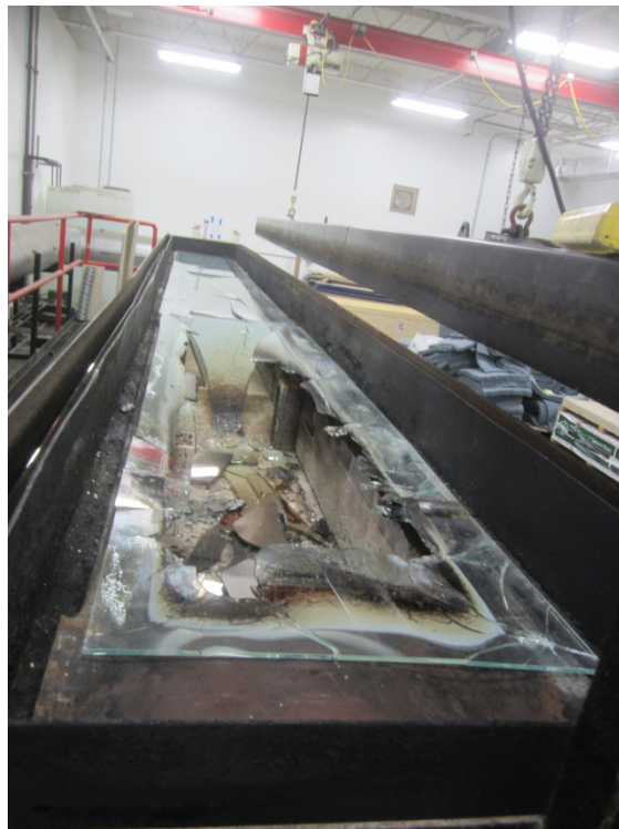
Photo No. 2 Unexposed Surface (Post-test) www.archtest.com
