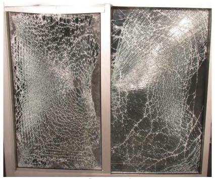
**Photo No. 95**Post-test Specimen #32, Interior
