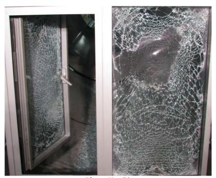
**Photo No. 50**Post-test Specimen #17, Interior
