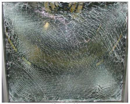
**Photo No. 29**Post-test Specimen #10, Interior
