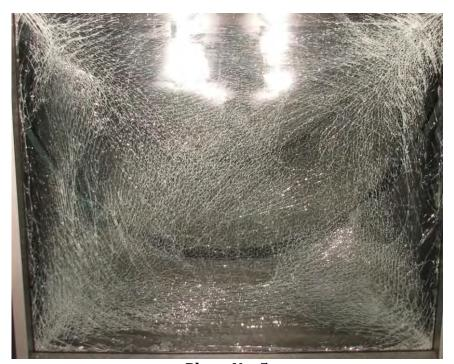
Photo No. 5 Post-test Specimen #2, Interior
