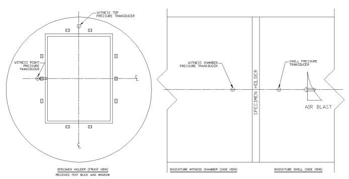
**Figure #2** Pressure Sensor Locations
