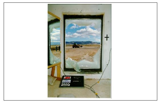
Figure A.88. Test 3. Posttest, interior view of window 1 (3M T3 POST 22.tif).
