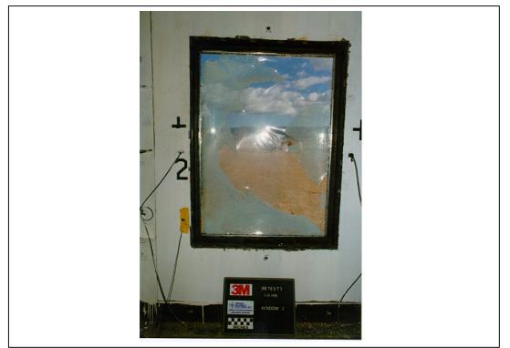
Figure A.95. Test 3. Posttest, interior view of window 2 (3M T3 POST 25.tif).
