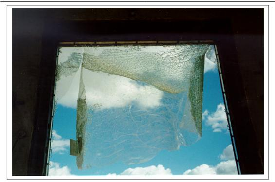
Figure A.101. Test 3. Posttest, interior view of window 3 (top half) (3m sd T3 post01.tif).
