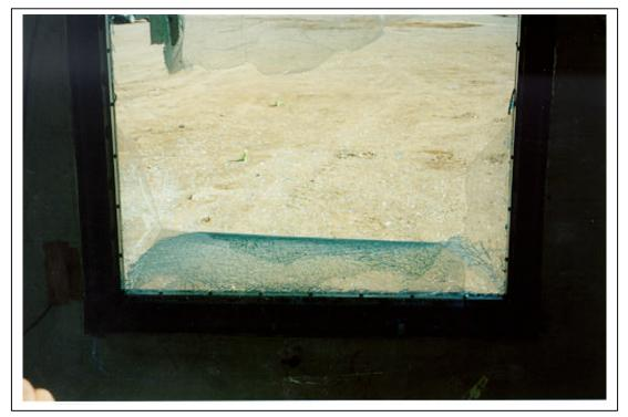
Figure A.102. Test 3. Posttest, interior view of window 3 (bottom half) (3m sd T3 post02.tif).
