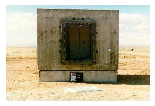
Figure 7.8. Exterior posttest view of window 4, test 5 (3M T5 post 37.tif).
