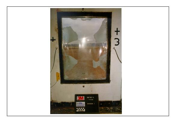
Figure A.199. Test 6. Posttest, interior view of window 3 (3M T6 POST 35. tif).
