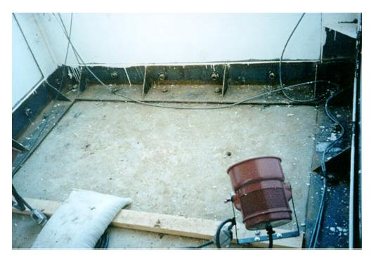
Figure 3.5. Interior view of glass fragmentation from window 2, test 1 (3M SD T1 post 18.tif).
