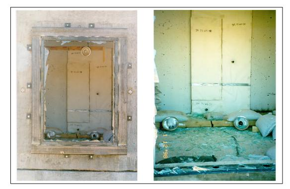
Figure A.43. Test 1. Posttest, exterior views of window 4 (3M T1 POST 11.tif, 3M T1 F58.tif).
