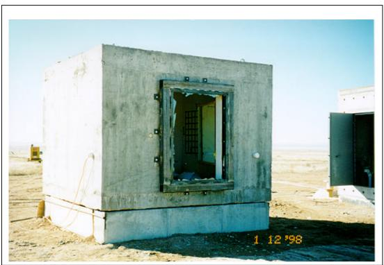
Figure A.42. Test 1. Posttest, exterior view of window 4 (3M T1 F61.tif).
