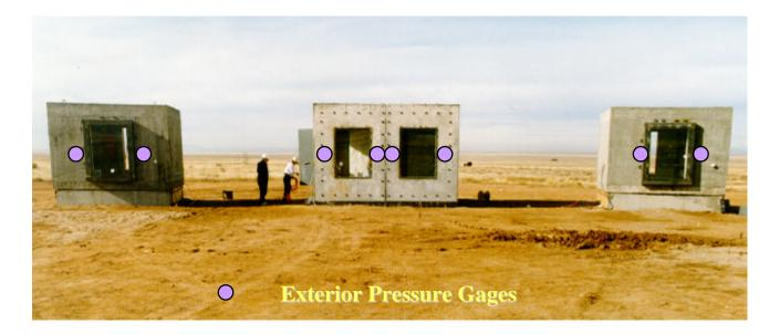
Figure 2.3. Exterior pressure gage locations.
