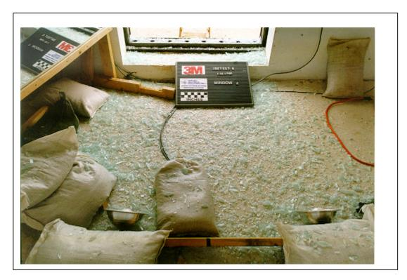
Figure A.212. Test 6. Posttest view of the South Structure floor (3M T6 POST 26.tif).
