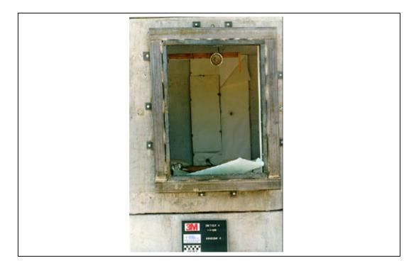
Figure A.109. Test 3. Posttest, exterior view of window 4 (3M T3 POST 16.tif).
