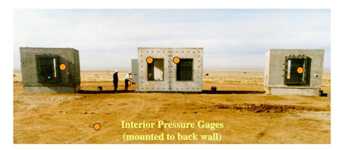
Figure 2.4. Interior pressure gage locations.
