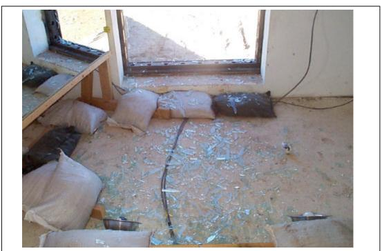
Figure A.45. Test 1. Posttest view of glass debris on the South Structure floor (test1\_42.jpg).
