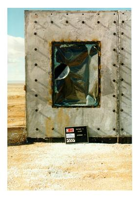
Figure 7.6. Exterior posttest view of window 3, test 5 (3M T5 post 32.tif).
