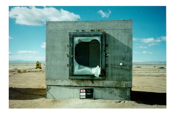
Figure 5.2. Exterior posttest view of window 1, test 3 (3M SD T3 post 24.tif).
