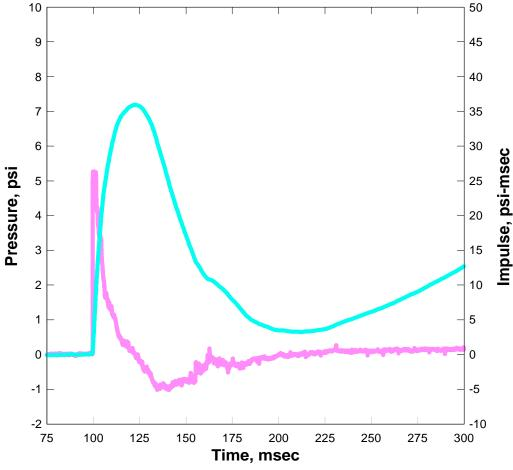
Figure 5.1. Typical airblast waveform from test 3.
