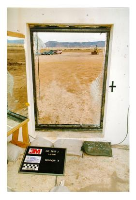
Figure 4.9. Interior view of glass fragmentation from window 4, test 2 (3M T1 post 20.tif).
