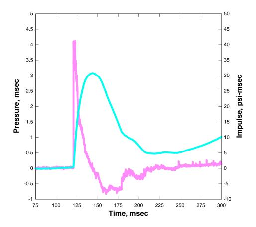
Figure 4.1. Typical airblast waveform from test 2.
