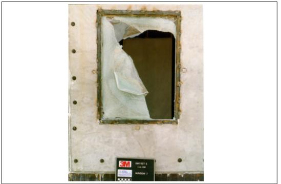
Figure A.193. Test 6. Posttest, exterior view of window 2 (3M T6 POST 02.tif).
