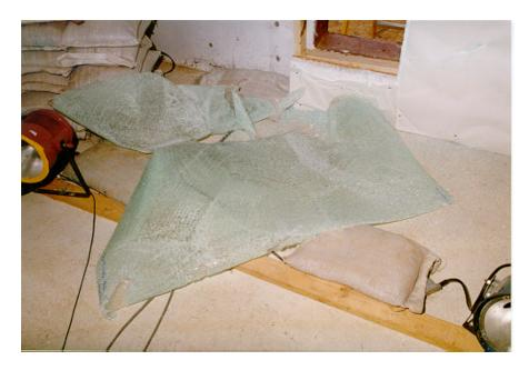
Figure 8.3. Interior posttest view of window 1 fragmentation near the rear of the structure, test 6 (3M T6 post 21.tif).
