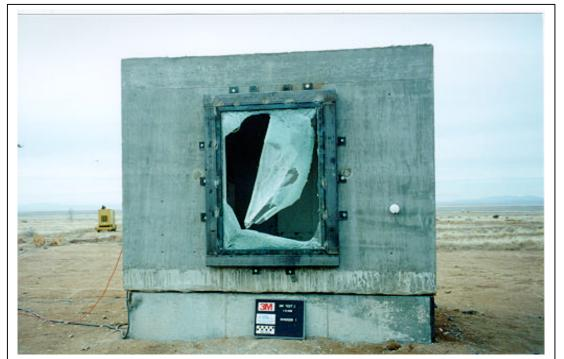
Figure A.55.Test 2. Posttest, exterior view of window 1 (3m sd T2 post27).
