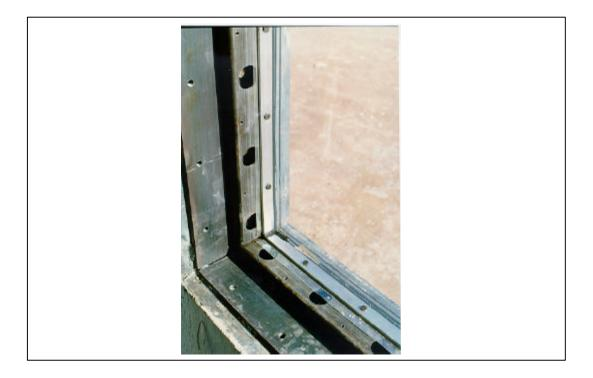
Figure A.92. Test 3. Pretest, interior view of window 1. Close-up view of the batten system (3M T3 PRE 05.tif).
