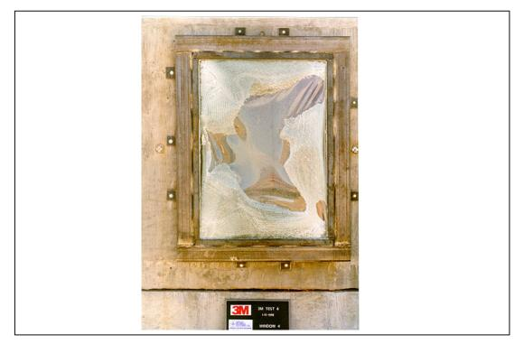
Figure A.144. Test 4. Posttest, exterior view of window 4 (3M T4 POST 32.tif).
