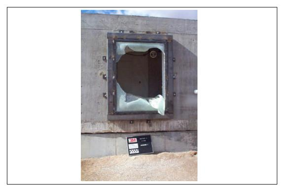
Figure A.87. Test 3. Posttest, exterior view of window 1 (test3\_23.jpg).
