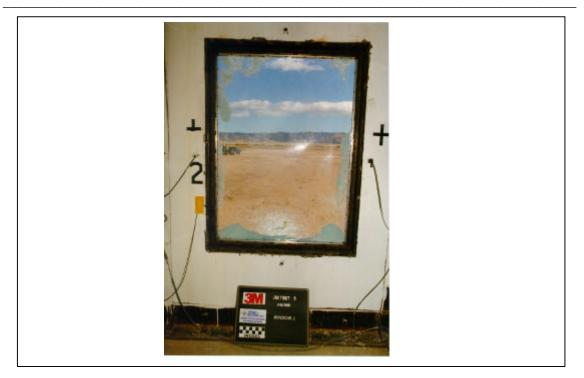
Figure A.161. Test 5. Posttest, interior view of window 2 (3M T5 POST 04.tif).
