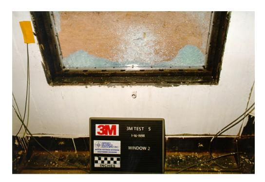
Figure 7.5. Interior view of window 2 frame deformation, test 5 (3M T5 post 06.tif).
