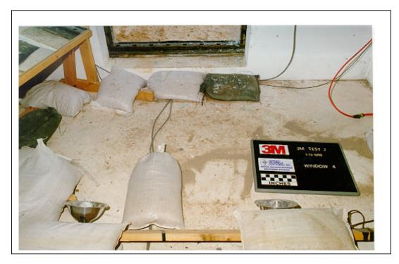
Figure A.80. Test 2. Posttest view of the glass debris on the South Structure floor (3M T2 POST 22.tif).
