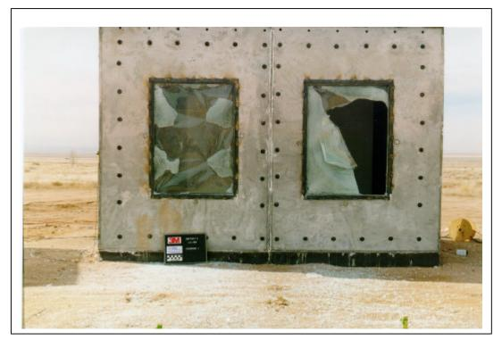
Figure A.192. Test 6. Posttest, exterior view of windows 2 and 3 (3M T6 POST 05. tif).
