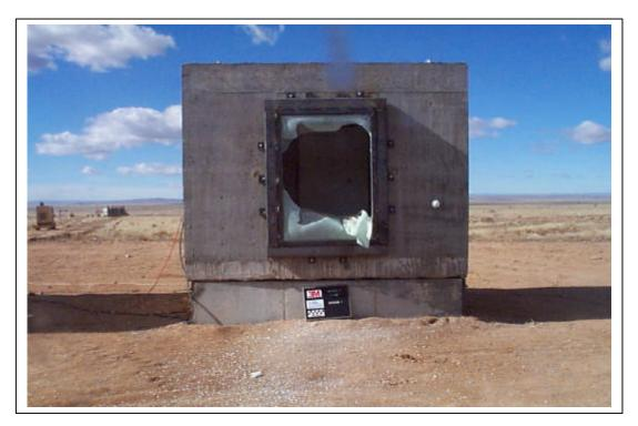
Figure A.86. Test 3. Posttest, exterior view of window 1 (test3\_22.jpg).
