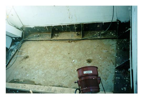
Figure 3.7. Interior view of glass fragmentation from window 3, test 1 (3M SD T1 post 31.tif).
