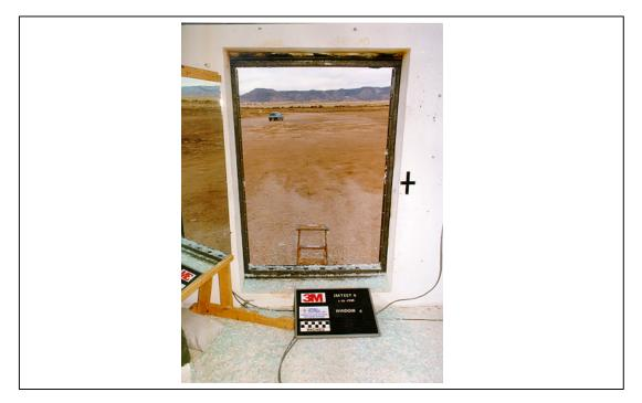
Figure A.210. Test 6. Posttest, interior view of window 4 (3M T6 POST 23.tif).
