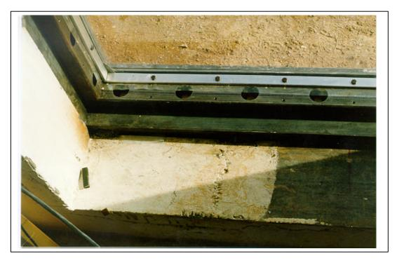
Figure A.61 Test 2. Pretest, interior view of window 2. Close-up view of the batten system (3M T2 PRE 09.tif).
