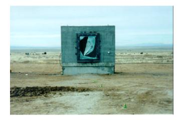
Figure 4.2. Exterior posttest view of window 1, test 2 (3M SD T2 post 45.tif).
