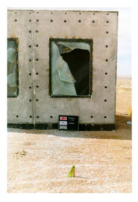
Figure 8.4. Exterior posttest view of window 2, test 6 (3M T6 post 01.tif).
