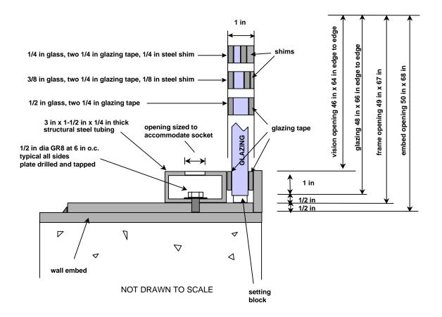
Figure 2.9. Glazing installation detail.
