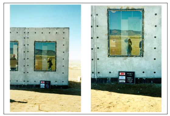
Figure A.25. Test 1. Pretest, exterior views of window 2 (3m sd T1 pre09.tif, 3m sd T1 pre08.tif).
