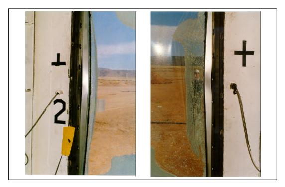
Figure A.130. Test 4. Posttest, interior views of window 2. Pictures of the aluminum frame displacement along the vertical edges (3M T4 POST 16.tif).
