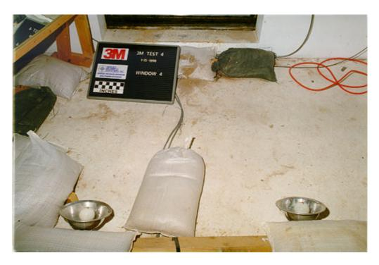
Figure 6.8. Interior view of window 4 fragmentation, test 4 (3M T4 post 45.tif).
