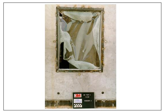
Figure A.63. Test 2. Posttest, exterior view of window 2 (3M T2 POST 17.tif).
