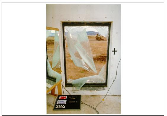
Figure A.57. Test 2. Posttest interior view of window 1 (3M T2 POST 12 .tif).
