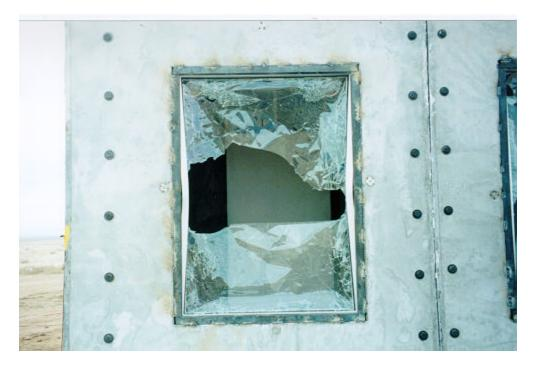
Figure 4.6. Exterior posttest view of window 3, test 2 (3M SD T2 post 37.tif).
