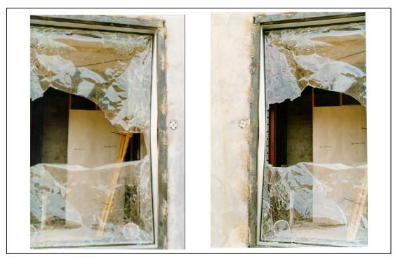
Figure A.70. Test 2. Posttest, exterior views of window 3 (3M T2 POST 37.tif, 3M T2 POST 38.tif).
