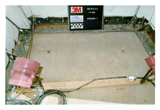
Figure 5.6. Interior view of window 3 and fragmentation, test 3 (3M T3 post 30.tif).
