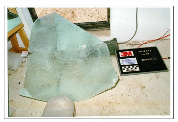
Figure A.111. Test 3. Posttest, interior view of window 4 (3M T3 POST 33.tif).
