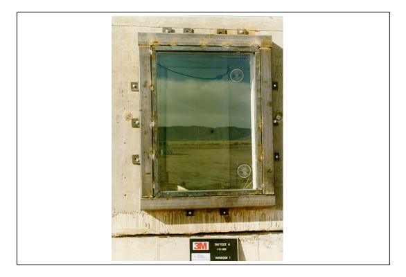
Figure A.116. Test 4. Pretest, exterior view of window 1 (3M T4 PRE 18.tif).
