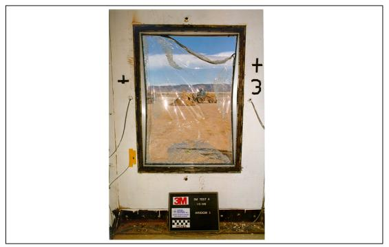
Figure A.137. Test 4. Posttest interior view of window 3 (3M T4 POST 30.tif).
