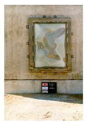
Figure 6.7. Exterior posttest view of window 4, test 4 (3M T4 post 44.tif).
