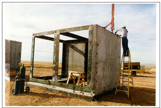
Figure A.2. The steel frame of the modular reaction structure (3M PREP 13.tif).
