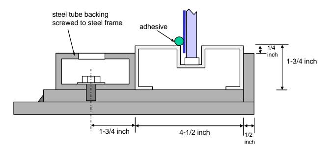
Figure 2.11. Aluminum frame mounting detail with a wet glazed film attachment.
