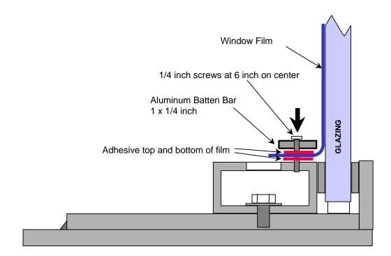
Figure 2.10. Film batten attachment detail.
