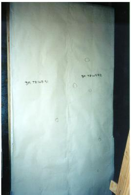
Figure 4.7. Interior view of witness panel impact from window 3, test 2. Impacts are circled (3M SD T2 post 06.tif).
