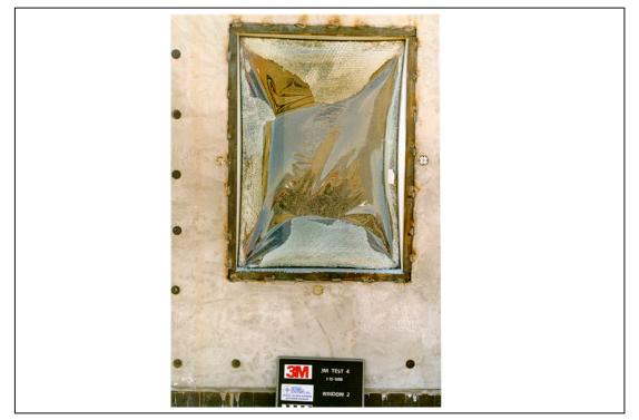
Figure A.128. Test 4. Posttest, exterior view of window 2 (3M T4 POST 11.tif).
