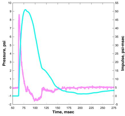
Figure 7.1. Typical airblast waveform from test 5.
