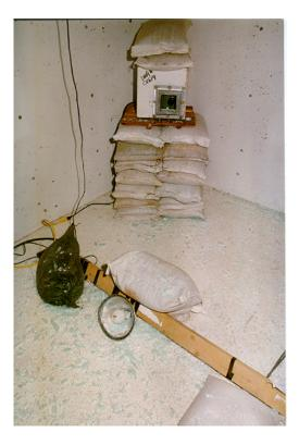
Figure 8.9. Interior view of window 4 glass fragmentation, test 6 (3M T6 post 29.tif).
