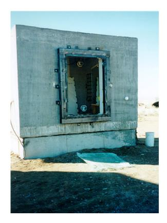
Figure 3.3. Exterior posttest view of window 1, test 1 (3M SD T1 post 05.tif).
