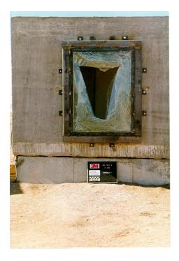
Figure 6.1. Exterior posttest view of window 1, test 4 (3M T4 post 06.tif).
