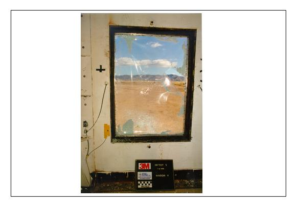
Figure A.166. Test 5. Posttest, interior view of window 3 (3M T5 POST 45. tif).
