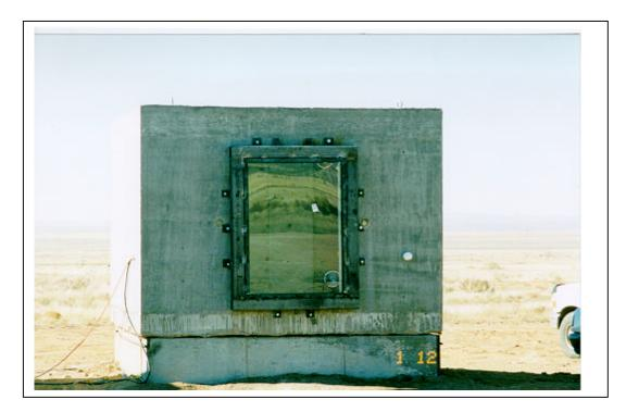
Figure A.11. Test 1. Pretest, exterior view of window 1 (3M T1 F26.tif).
