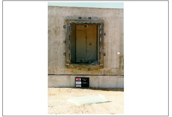
Figure A.175. Test 5. Posttest, exterior view of window 4 (3M T5 POST 38.tif).
