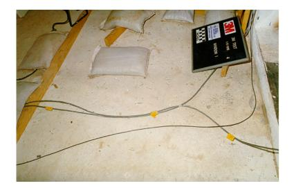
Figure 6.2. Interior view of fragmentation from window 1, test 4 (3M T4 post 20.tif).
