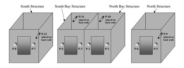
Figure B.1. Illustration of pressure gauge locations.
