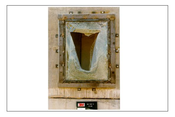
Figure A.120. Test 4. Posttest, exterior view of window 1 (3M T4 POST 05.tif).
