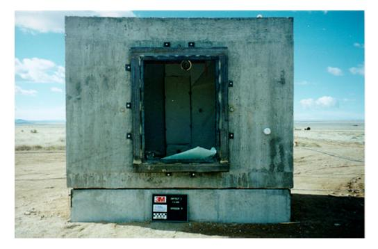
Figure 5.7. Exterior posttest view of window 4, test 3 (3M SD T3 post 14.tif).
