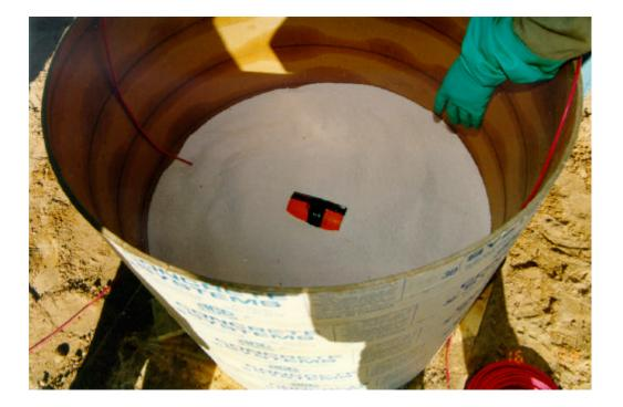
Figure 2.7. Pentolite booster in the center of the charge.
