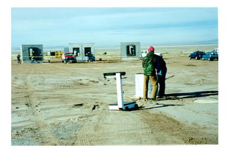
Figure 2.8. Technicians measuring charge standoff distance.
