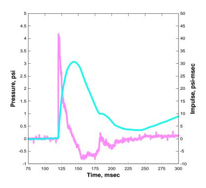
Figure 3.1. Typical airblast waveform from test 1.
