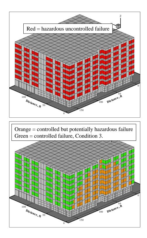
Figure 9.1. Damage comparison calculations: top calculation = no film; bottom calculation = film retrofits.
