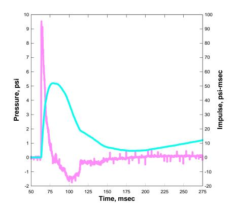
Figure 8.1. Typical airblast waveform from test 6.
