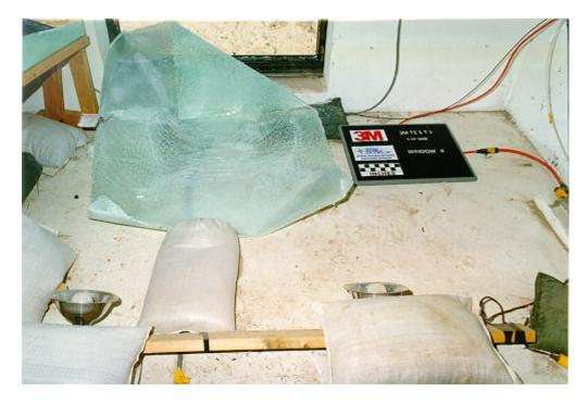
Figure 5.8. Interior view of window 4 and fragmentation, test 3 (3M T3 post 01.tif).
