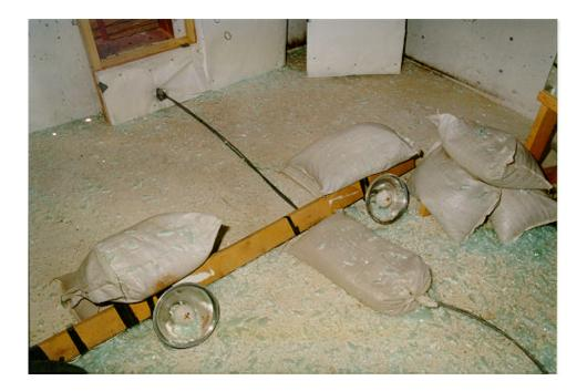
Figure 8.8. Interior view of window 4 glass fragmentation, test 6 (3M T6 post 27.tif).
