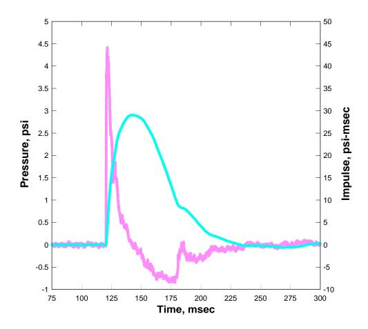
Figure 6.1. Typical airblast waveform from test 4.
