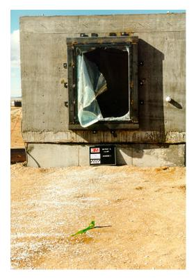
Figure 7.2. Exterior posttest view of window 1, test 5 (3M T5 post 25.tif).
