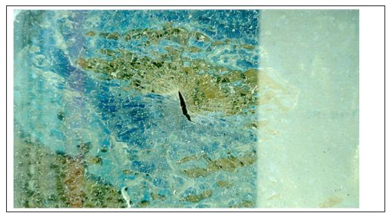
Figure A.168. Test 5. Posttest, exterior view of window 3. Picture of an apparent projectile penetration (3M sd T5 post01.tif).
