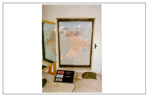
Figure A.145. Test 4. Posttest, interior view of window 4 (3M T4 POST 31.tif).
