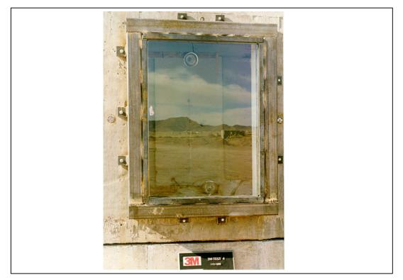
Figure A.140. Test 4. Pretest, exterior view of window 4 (3M T4 PRE 10.tif).
