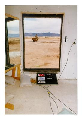
Figure 8.2. Interior posttest view of window 1 fragmentation near the front of the structure, test 6 (3M T6 post 19.tif).
