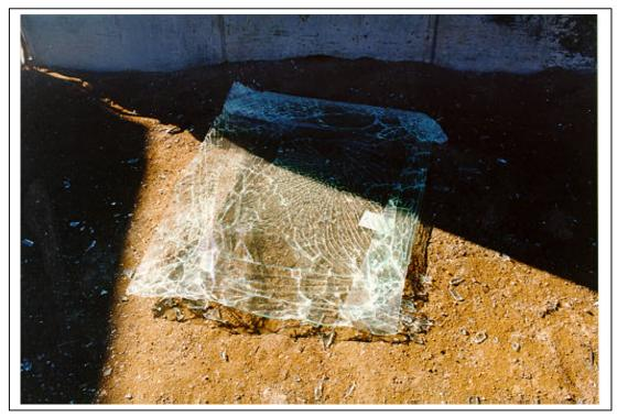
Figure A.19. Test 1. Posttest view of the security film and attached glazing from window 1 (3M T1 POST 05.tif).
