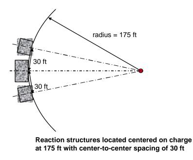
Figure 2.2. Radial orientation of structures (not drawn to scale).
