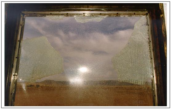
Figure A.201. Test 6. Posttest, interior view of window 3 (view of top half) (3M T6 POST 38.tif).
