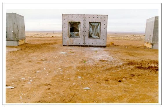
Figure A.62. Test 2. Posttest, exterior view of windows 2 and 3 (3M T2 POST 01.tif).
