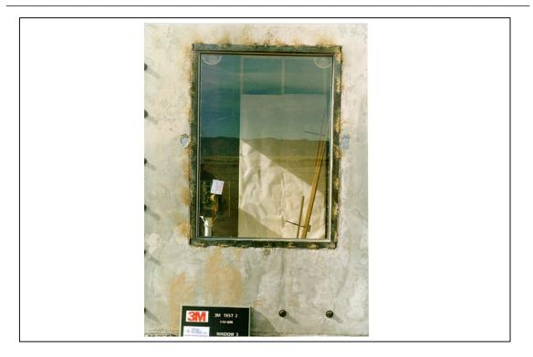
Figure A.66. Test 2. Pretest, exterior view of window 3 (3M T2 PRE 17.tif).
