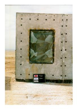
Figure 8.6. Exterior posttest view of window 3, test 6 (3M T6 post 04.tif).
