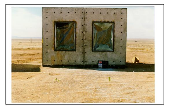
Figure A.127. Test 4. Posttest, exterior view of windows 2 and 3 (3M T4 POST 09.tif).
