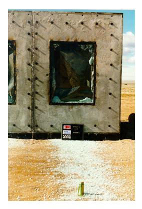
Figure 7.4. Exterior posttest view of window 2, test 5 (3M T5 post 28.tif).
