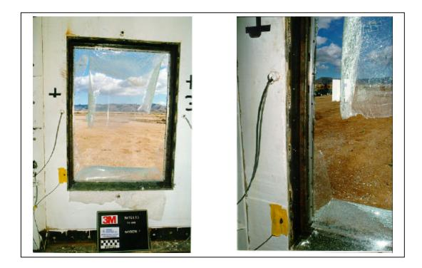
Figure A.100. Test 3. Posttest, interior views of window 3 (3M T3 POST 29.tif, 3M T3 POST 31.tif).
