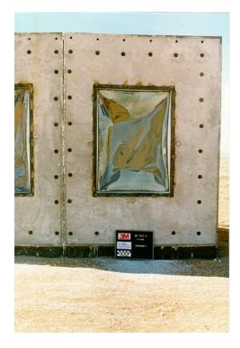
Figure 6.3. Exterior posttest view of window 2, test 4 (3M T4 post 10.tif).
