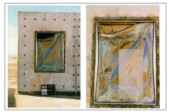
Figure A.136. Test 4. Posttest, exterior view of window 3 (3M T4 POST 41.tif, 3M T4 POST 33.tif).
