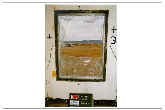
Figure A.71. Test 2. Posttest, interior view of window 3 (3M T2 POST 26.tif).
