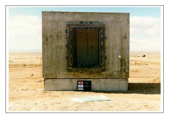
Figure A.174. Test 5. Posttest, exterior view of window 4 (3M T5 POST 37. tif).
