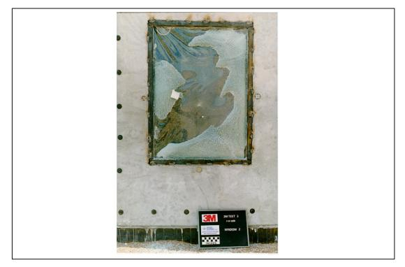
Figure A.94. Test 3. Posttest, exterior view of window 2 (3M T3 POST 10.jpg).
