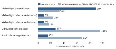
All performance results are based on the film installed on the inside surface of 1/8" (3mm,) 1/4" (6mm,) and 1/8"+1/8" (3mm+3mm) thick, clear glass.
