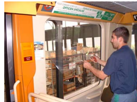
Graffitigard film is easily peeled away when it is vandalized, allowing professional installers to quickly apply a fresh layer.
